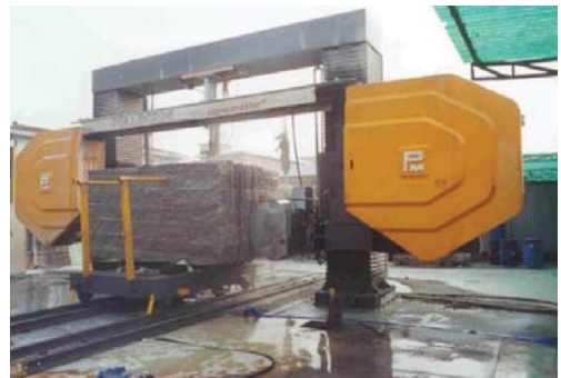
Fig. 3 Stationary machine for stone cutting wire
