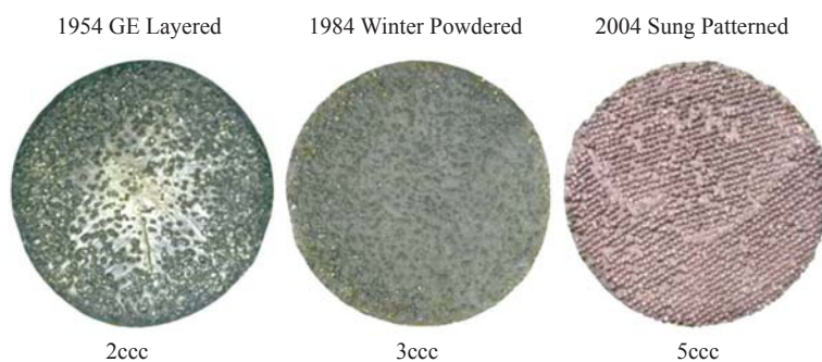
Fig. 1 The three cell designs for growing saw diamond and their optimized yields in carat per cubic centimeter (ccc) of compressed cells. These cells were pressed at Huanghe Whirlwind in 2003.
